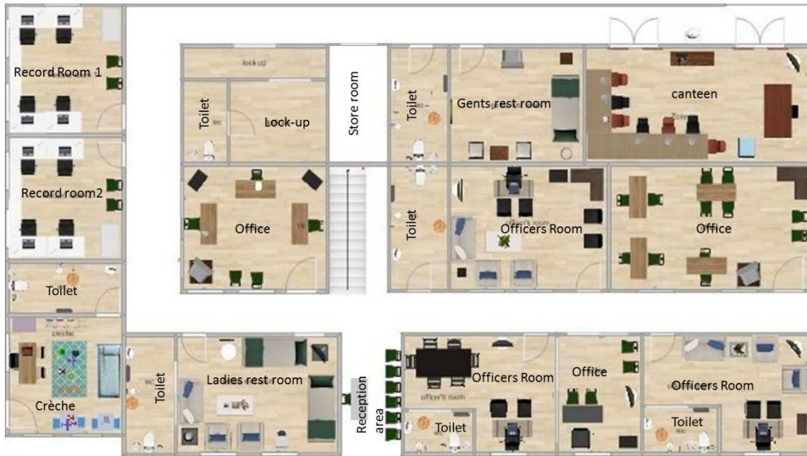
Figure 2: Design layout of a Pan Bazar police station along with arrangement of furniture, fittings and fixtures
