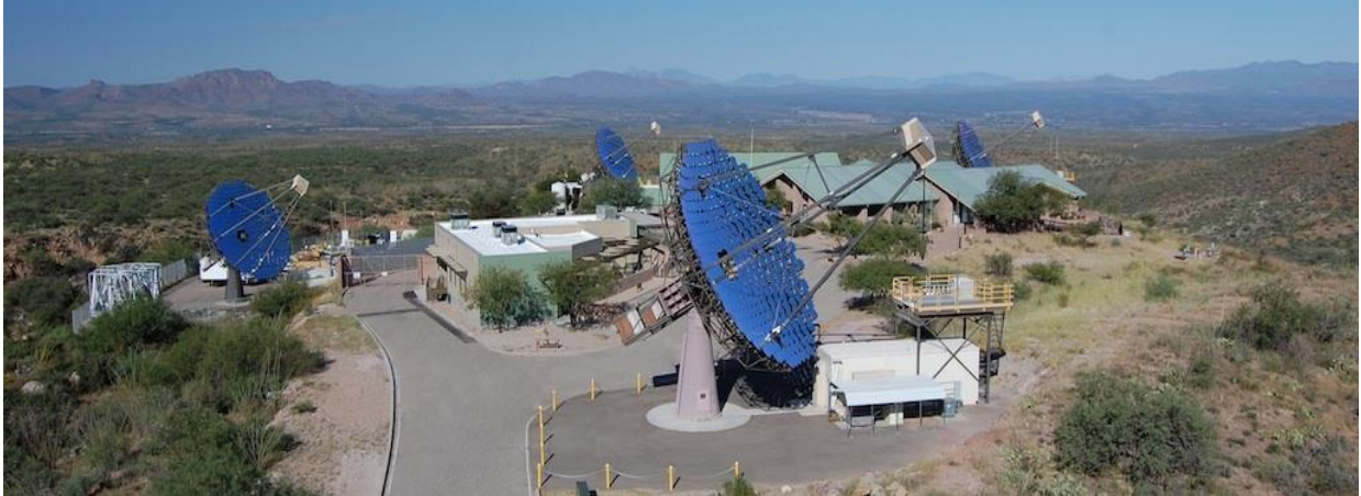
Figure 4: This is an image of the VERITAS gamma ray observatory, which operates at the Fred Whipple Observatory (FLWO) base camp in Tucson, AZ. Seen in the image are the four individual 12-meter telescopes and the facilities that help run the telescopes. Retrieved from https://veritas.sao.arizona.edu/
