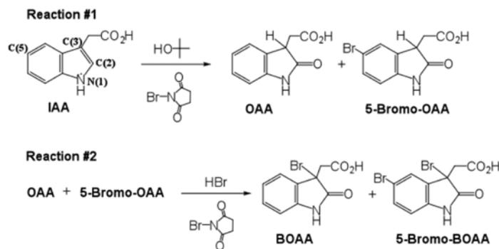
To test the two-step reaction scheme proposed in Figure 6, we ran the traditional BOAA synthesis from IAA by adding NBS in two separate steps. The results of these reactions (data not shown) clearly show that addition of one mole equivalent of NBS produces OAA and 5-bromo-OAA. Subsequent addition of a second NBS mole equivalent gives the typical product distribution shown in Figure 5.
