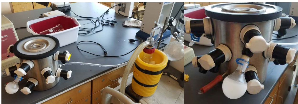
Figure 8. Lyophilizer used to dry the GSMOI.
