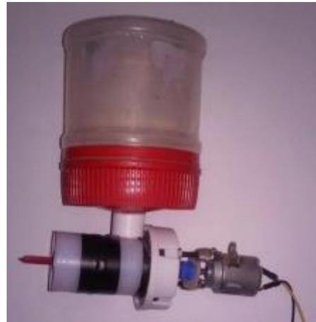
The radio receiver will send a PWM signal, a servo motor, that activates or deactivates the motor to start the process of seed dispensing.
